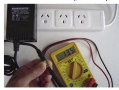
If there's an intermittent fault in the cable, flexing the cable – particularly from where it emerges from the plug pack and enters the connector – will cause the reading on the meter to jump around. If this happens, you know you have a dodgy lead.
