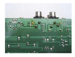
If you've found a dry joint and you intend to fix it yourself, it's best to clean off any existing solder first by using either a de-soldering tool or solderwick before re-soldering anything. There's lots of information available on the web on solder tips and techniques, so look them up.
