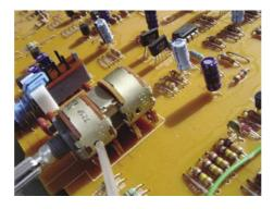
Likewise, access to switches for cleaning varies, but due to the penetrating nature of spray contact cleaners, it's usually possible to get cleaner into the mechanism. Once again, toggling the switch a number of times immediately after squirting in the cleaner is important – don't forget: the cleaner needs you to work with it to affect a solution!
